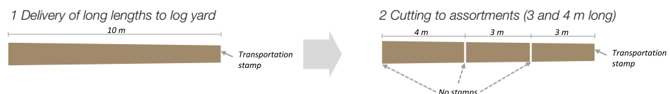
Figure 7: Exemplary scheme of cutting long lengths to assortments at a log yard
