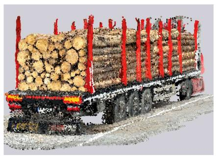
Picture 9. LiDAR image for volume measurement
