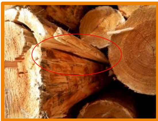
Crack on the lateral surface
