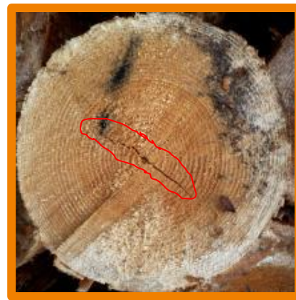
Superficial frontal core crack
