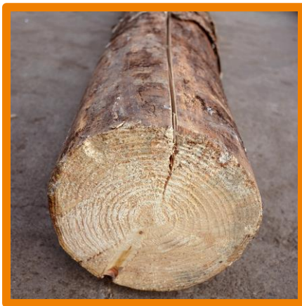
Crack on the lateral surface
