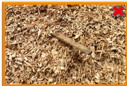
Unsuitable Chips, inappropriate objects
