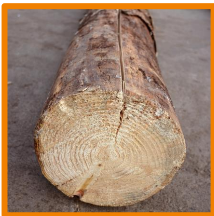
Crack on the lateral surface
