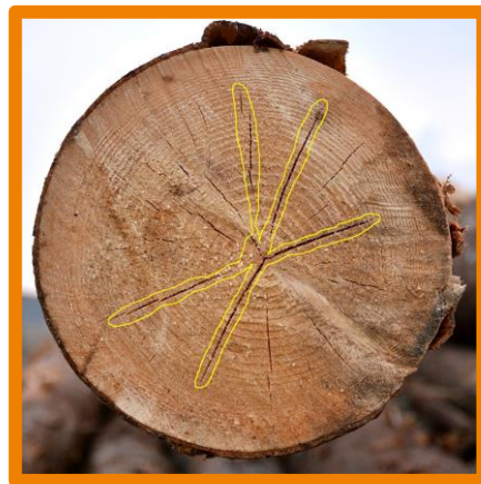
Superficial frontal core crack
