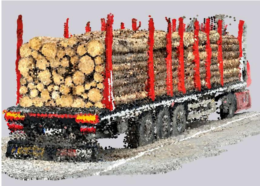
Picture 9. LiDAR image for volume measurement
