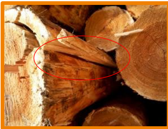
Crack on the lateral surface
