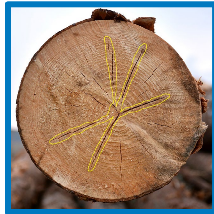
Superficial frontal core crack
