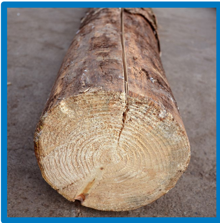
Crack on the lateral surface
