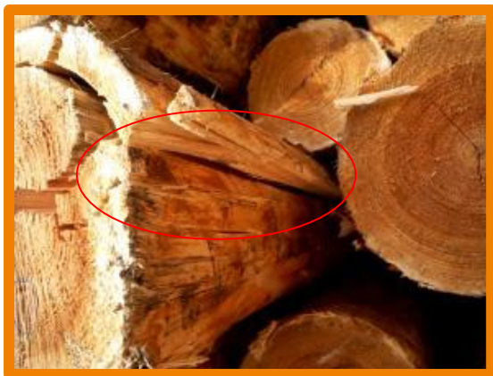
Crack on the lateral surface
