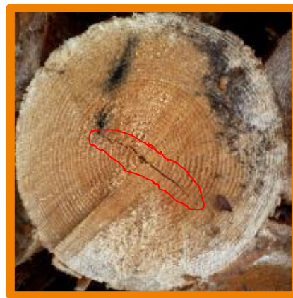
Superficial frontal core crack
