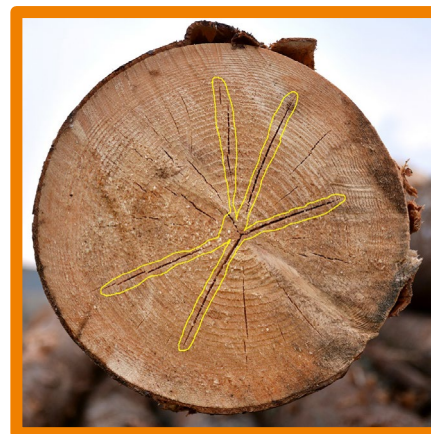
Superficial frontal core crack
